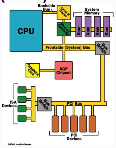
This illustration shows how the various buses connect to the CPU.
